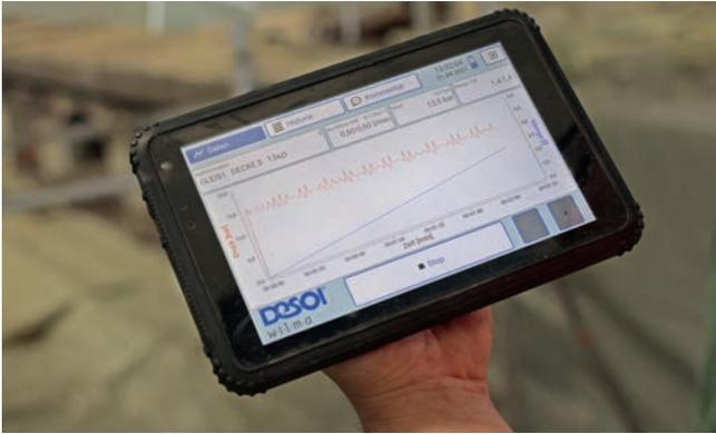
Desoi w.i.l.m.a. records the pressure, volume, time and any deviations of the injection processes
