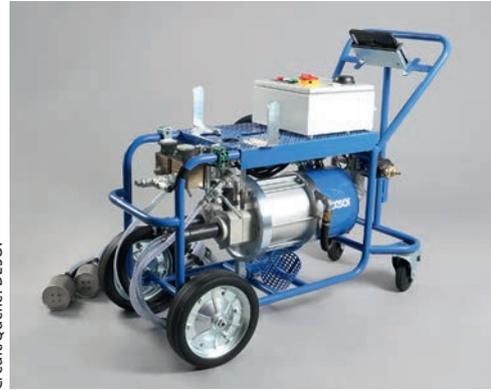
Recording and documentation system w.i.l.m.a.-PU for polyurethane and silicate resin
